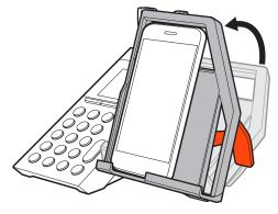
2 To release the charge platform, pull the orange lever forward.
