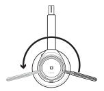
**TIP** Your headset senses when you change the microphone boom from one side to the other and syncs the audio and controls specific to each side.
