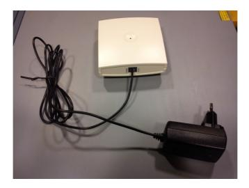
Power supply for the repeater is 9VDC, 300mA.
